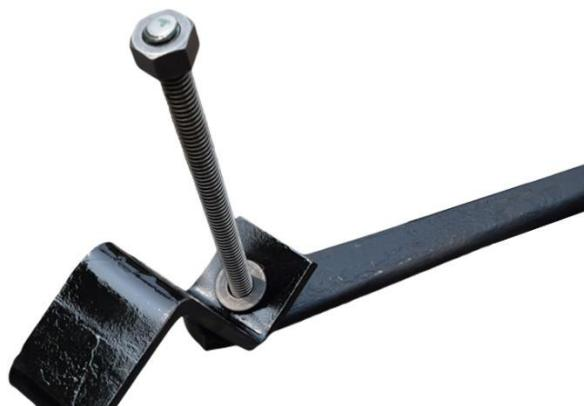
**Step 8b:** Insert the 5/8" Acme bolts through the bottom of the springs and then through the bottom of the spring tensioning brackets. Place the spherical washer with the convex side down onto the 5/8 acme bolt. Screw an acme nut onto the bolt with no more than a single thread protruding out of the top of the nut.
