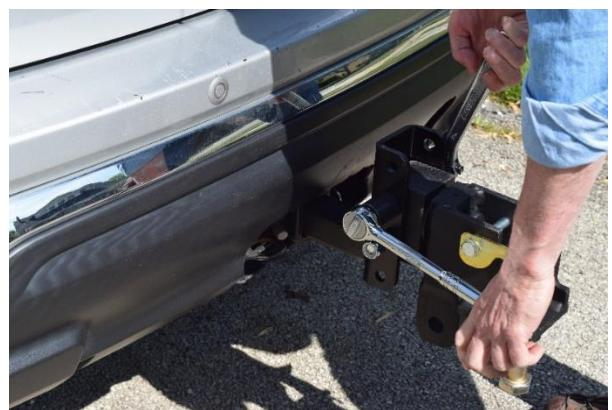
**Step 4.** Before hitching the trailer, pick a spot that is easy to measure from on the vehicle such as the center of the rear wheel well or the top of the height adjustment channel. Record the distance from the ground to your chosen point.
