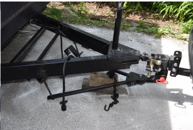
**Step 11.** Place the spring tensioning brackets on the trailer frame and screw the 1/2" bolts into the spring tensioning brackets. Don't tighten them yet. Just bring them close to the frame.
