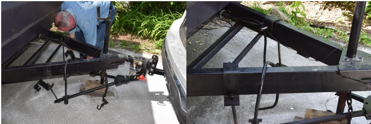
**Step 12.** Raise the spring bars up by using the 5/8" acme bolt & nuts. . Adjust the 1" angle adjustment bolt up or down to create the right distance. There should be 6-8" of gap between the springs and the bottom of the trailer frame. At this point in the procedure the 1" bolt should be tight against Item 3. NOTE: If you are compensating for a heavy load it is better to start with the larger 8" gap.
