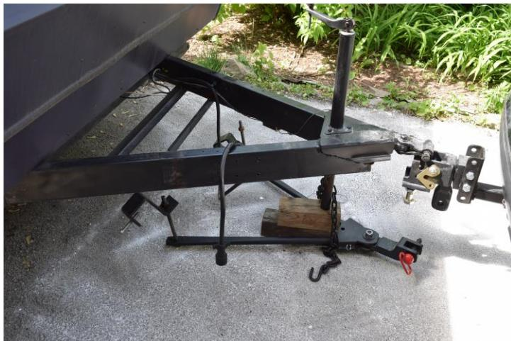
**Step 10.** Using the provided 7/8" dia. hitch pin or a 7/8" bolt, attach the spring bar assembly to the vehicle side hitch.
