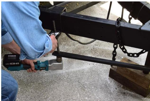
**Step 13.** Using the 1-1/16 socket on the bolt head and an adjustable wrench or open end 1-1/16 wrench on the nut, start to put tension on the springs. Alternate between the two sides. Tighten the 5/8 inch Acme bolts until there is a gap of 3 to 4 inches between the springs and the bottom of the trailer frame. A right angle impact wrench makes this much easier.
