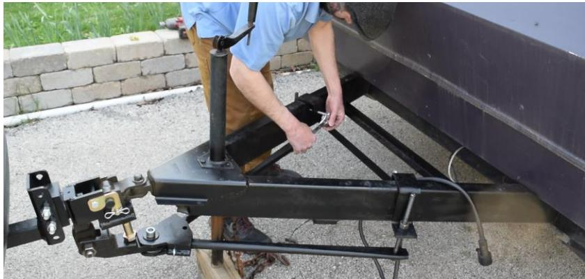
**Step 15.** Raise the jack back up and remeasure like in step 4. This value should be equal to or no more than 7/8" less than the value found in step 4.
